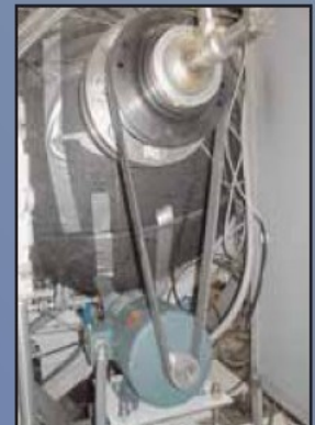
Belt-driven mixer using Co-Axial Type Coupling
